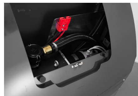
Battery and vacuum pump are integrated in the unit, protected by a robust cover.
