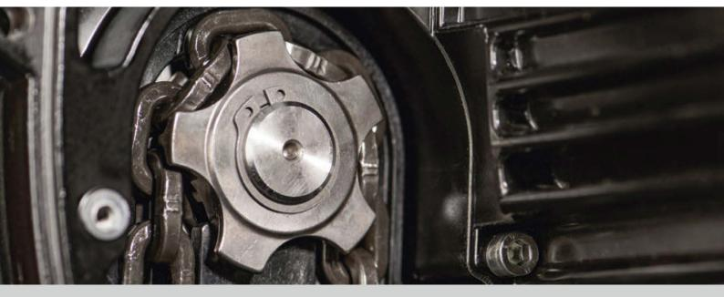
The GP series has an overall modular structure. Wearing parts are replaced in a simple manner. The electric chain hoist can be quickly disassembled and reassembled without special tools thanks to the polygonal connection. This saves time and costs, which both service technicians as well as customers appreciate.
